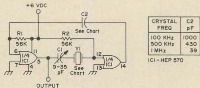
Crystal oscillator calibrator, high in square wave output (which means you will be able to hear it up into the VHF bands), which may be made into two calibrators since the circuit uses only half of the IC. This circuit appeared originally in HMA-36, Radio Amateur's IC Projects by Motorola, available free by writing Department 73, Box 20924, Phoenix AZ 85034.
