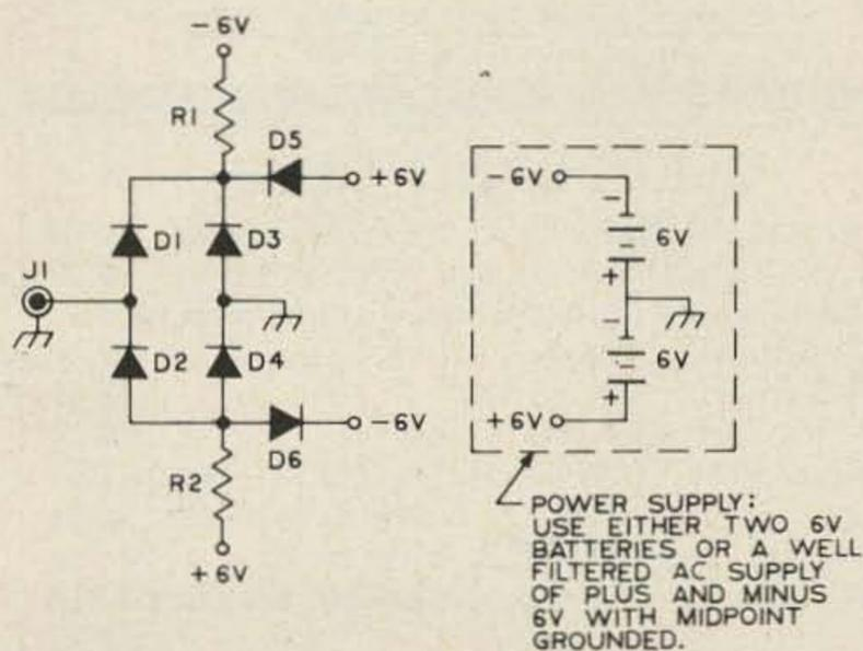
Fig. 1. A simple diode switch circuit using 6 diodes.
