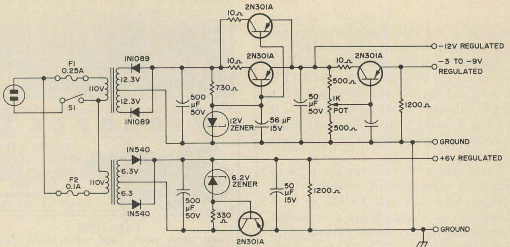
Fig. 17. Regulated power supply.
