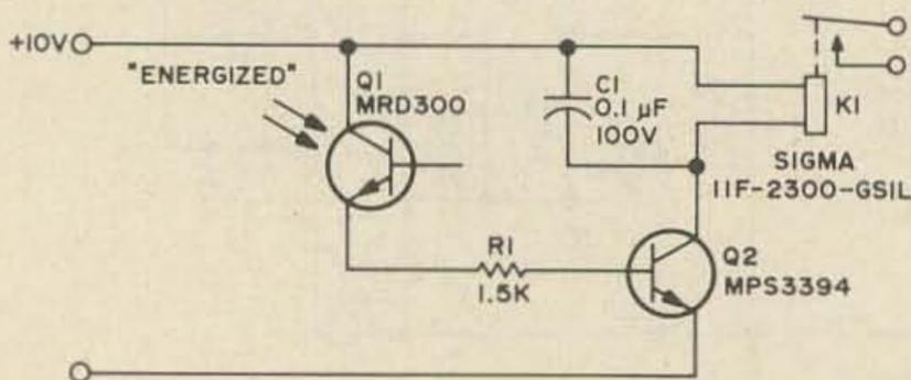
Light operated relay. It takes 220 foot candles to turn this on. Turning off the light turns off the relay. Circuit courtesy Motorola Semiconductor Power Circuits Handbook.
