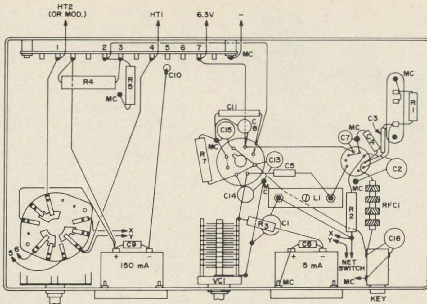
Fig. 3. Under the chassis.
