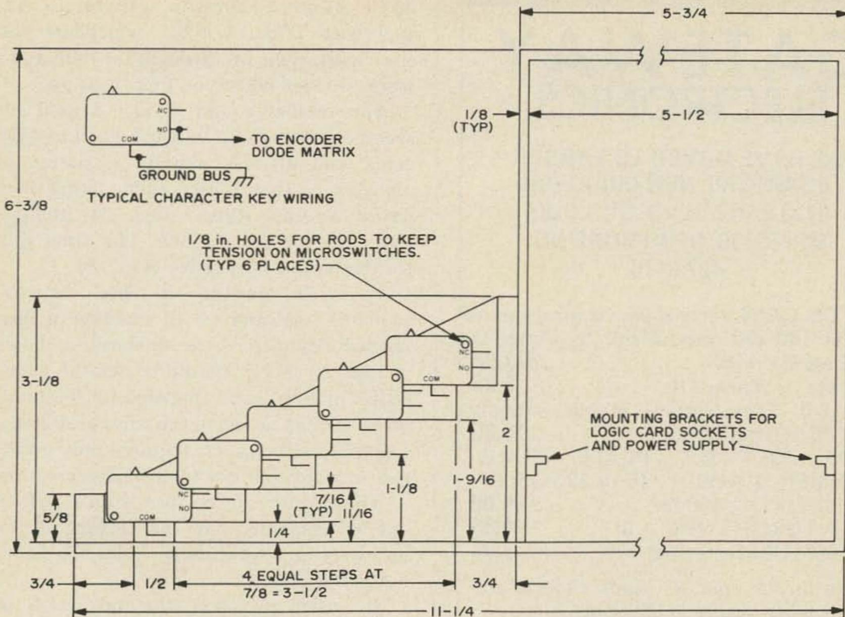
Fig. 20. Side view of button box, with dimensions.
