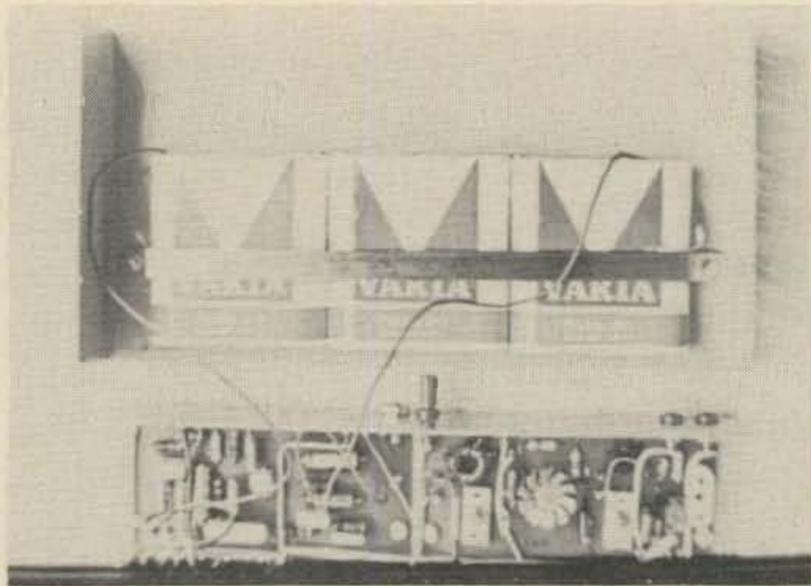
The power supply for the author's portable transceiver consists of three 4.5V flat batteries held in the top cover of the transceiver enclosure.
