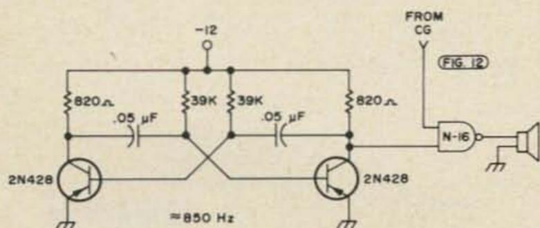
Fig. 19. Monitor oscillator.
