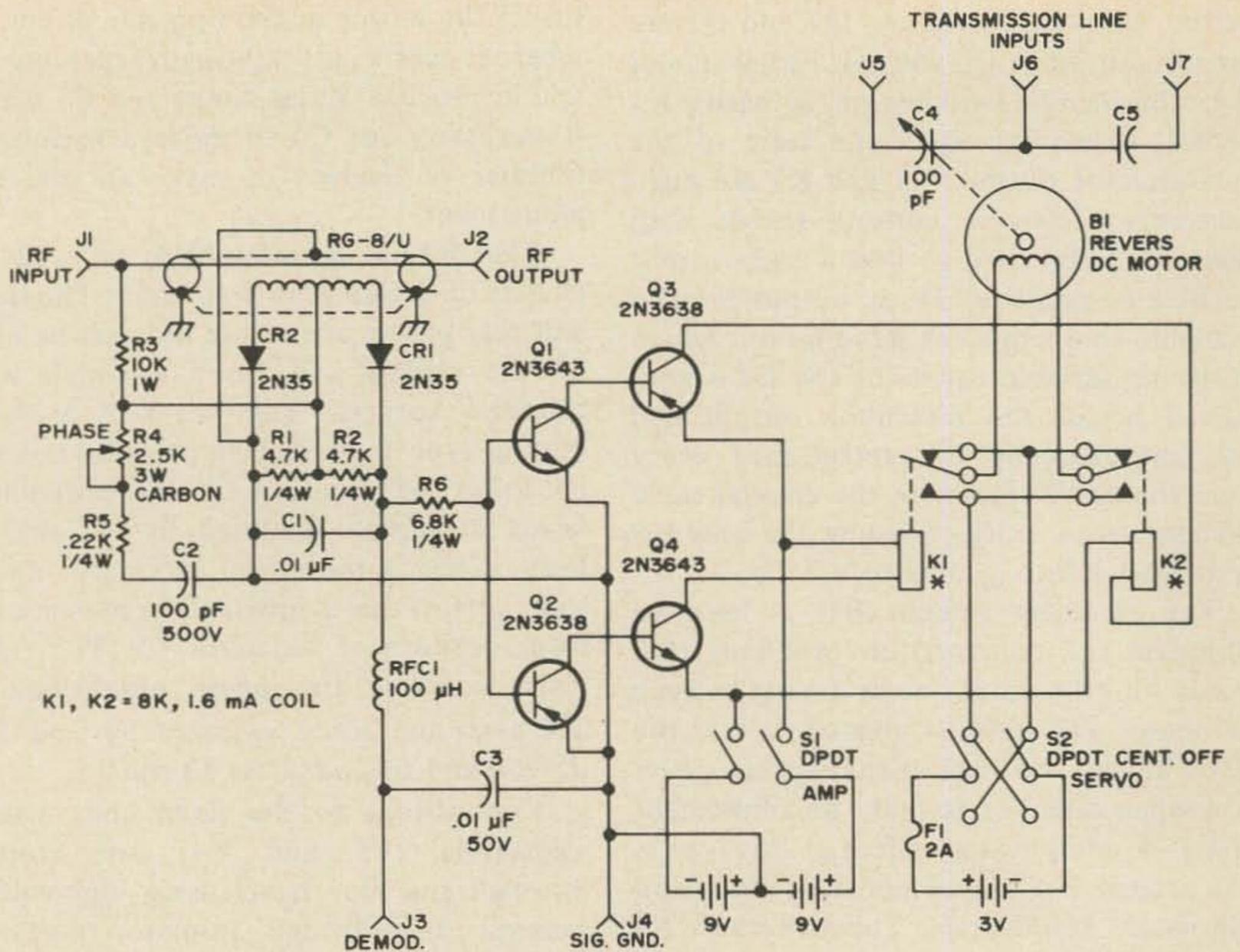
Fig. 2. Schematic - ATLT Unit
