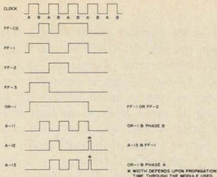
Fig. 11. Timing signals for button-box logic elements.
