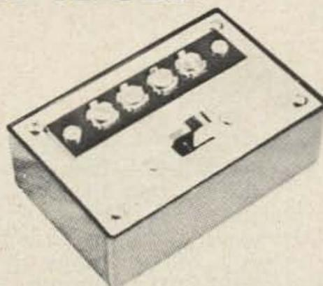
400 HZ active filter simply connected to speaker output and to a pair of headphones (8Ω to 2 KΩ) requires 9V battery, not included.
