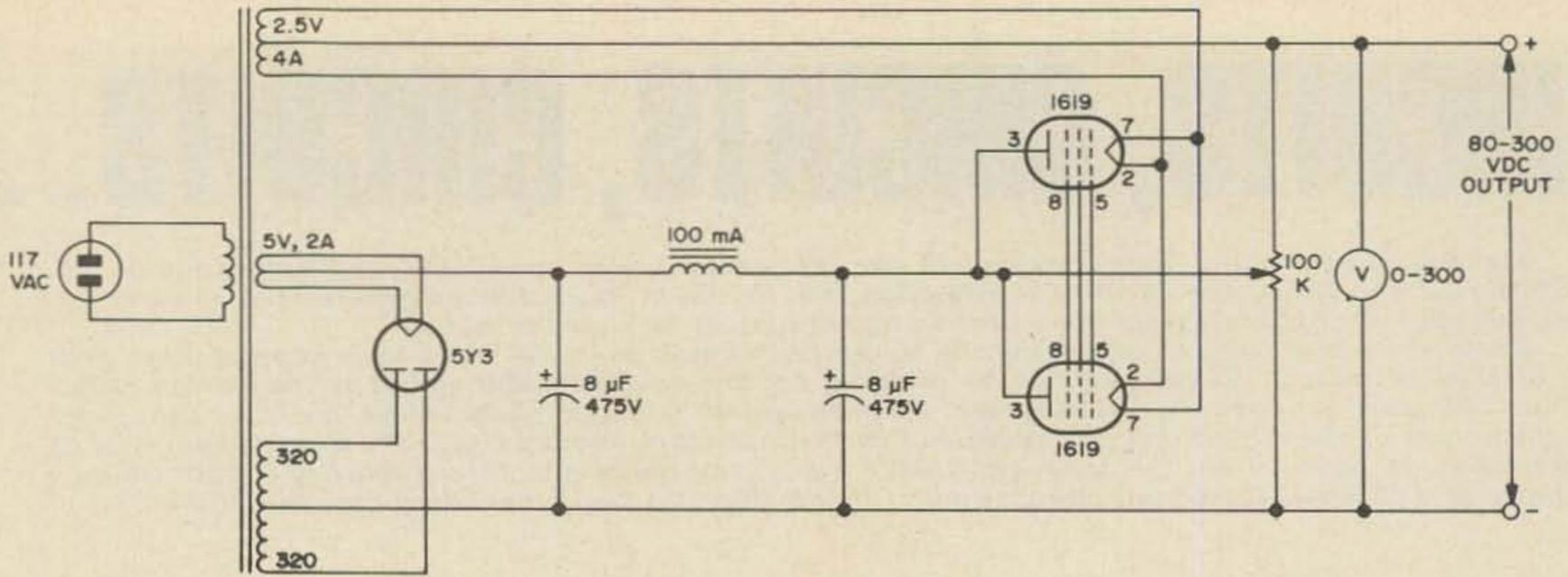
Variable power supply. Here's an oldie but goodie submitted by W4IOI and taken from a 20-year-old Heath flyer. If you keep in mind the filament requirements you can use 6L6s, 6Y6s, 1619s, 807s, 1625s, 837s, etc.
