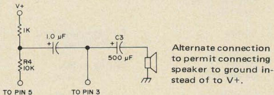
Typical circuit for a 1-watt audio power amplifier, using Motorola's Functional Circuit MFC8010. Circuit and data from Motorola's Functional Circuits book of application notes.
