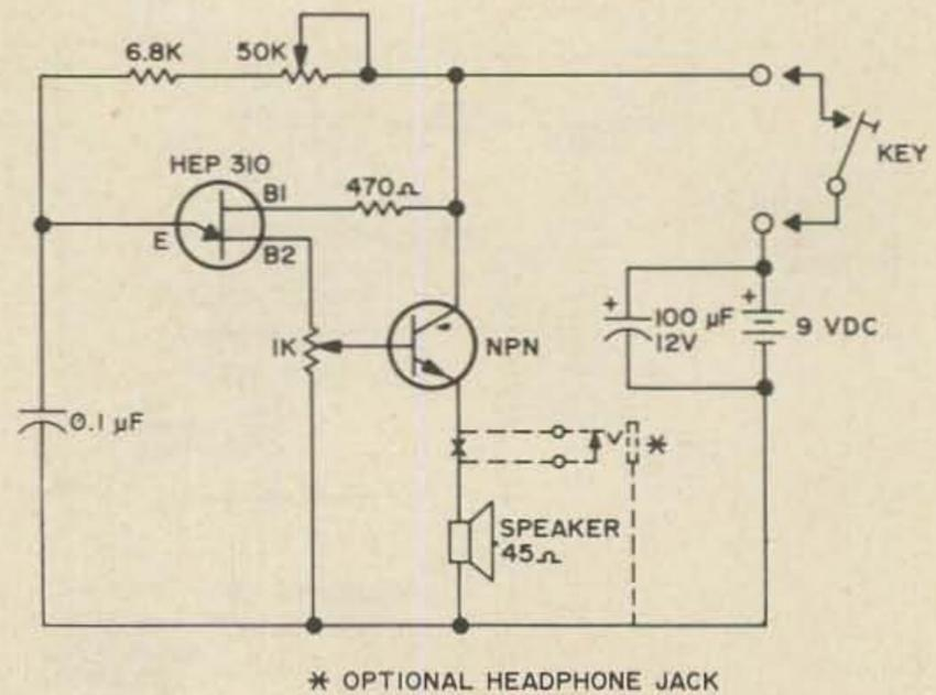
Code practice oscillator or perhaps a noisy alarm for the home, boat or car. Circuit courtesy Calectro Handbook (\$.50, GC Electronics, 400 S. Wyman, Rockford IL 61101). NPN transistor is a Calectro #K4-506.
