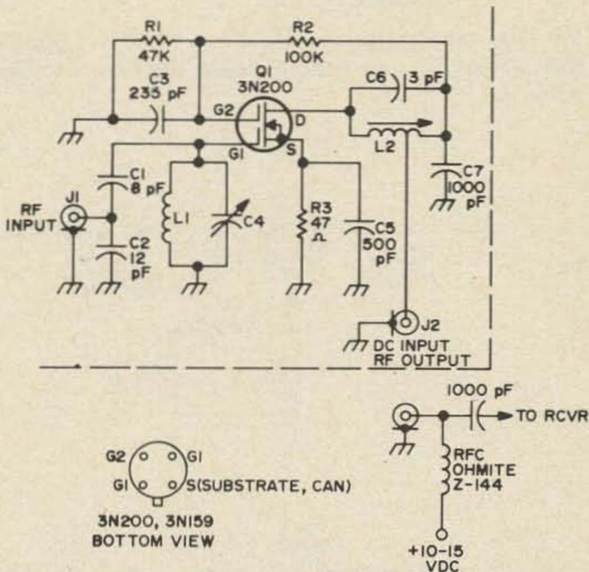
Two meter preamplifier, MOSFET. C4-5 are button picas and support transistor leads forming resonant circuit. L1 is JFD LC374 tank circuit which contains C1. L2 is 6T #22 enamel on 5 mm slug-tuned form, tap at 1 turn. 3N159 will also work in circuit. Circuit courtesy of RTTY Journal, P.O. Box 837, Royal Oak MI 48068. Circuit by W8BBB.
