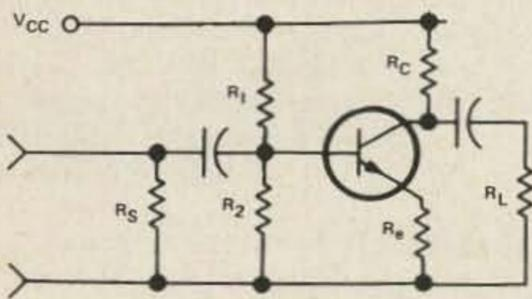
**Problem:** design an amplifier that will put out 10V peak to peak into a 10 k $\Omega$  load. A gain of 5 and an input impedance of 75 $\Omega$  are required.
