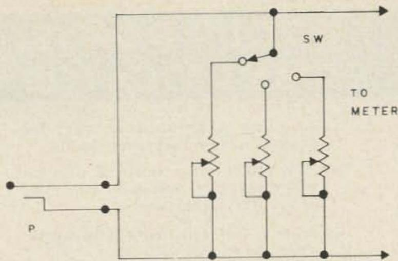
20Ω or SMALLER POTENTIOMETERS or FIXED RESISTORS
