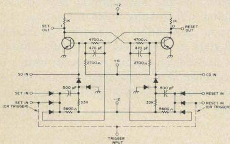
Fig. 16. Typical flip-flop.
