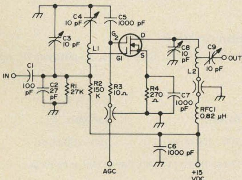
VHF amplifier used to measure gain, noise figure and AGC performance of the Fairchild FT0601 MOSFET. For AGC operation, dual-gate MOSFETs have a built-in advantage owing to their separate gates, especially in the VHF region. Amplifiers such as this one eliminate cross-modulation distortion, decrease receiver noise and avoid shifting of the receiver's center frequency. Schematic from Fairchild Semiconductor Application Note APP-189.
