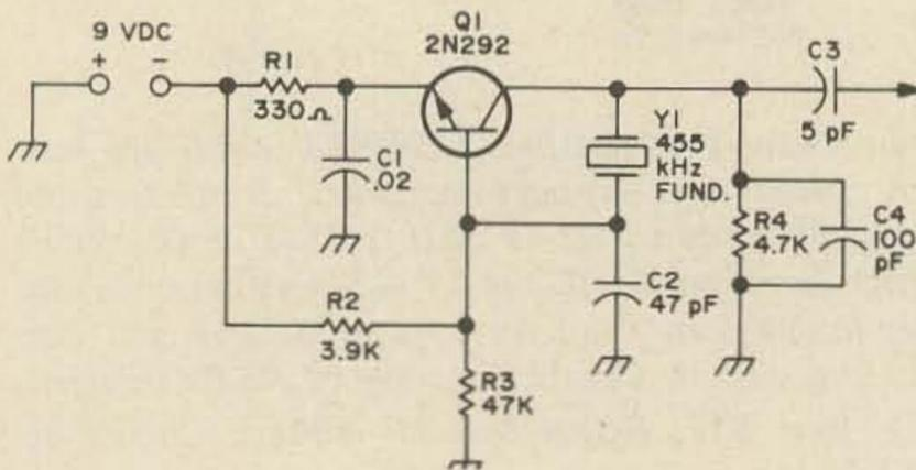
Two oscillator circuits for aligning receivers, anonymously presented, originally, in FM Bulletin, Vol. I, No. 5, June 1967, reprinted in 73's "FM Anthology I," available from 73 Magazine for \$3.00.
