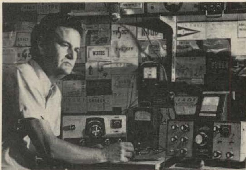
WB4SNC, Albert Coya, at his shack. The equipment is a HW-101 Heathkit, a HW 32 monobander for 20 meters, and a homebrew linear. Other gear shown: homebrew phone patch, frequency counter, keyer, SW R meter, monitor scope, and power supply for both rigs.
