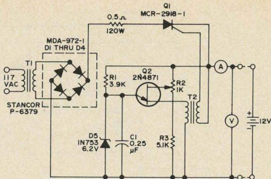
Foolproof Battery Charger. T2 is a Sprague 11Z12. Protects battery against overcharging or reverse charging, also protects itself against shorting or hurting another supply. Will supply 16A. Circuit courtesy Motorola Semiconductor Power Circuits Handbook.
