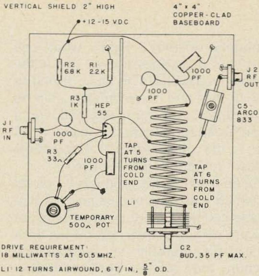
Fig. 7. Layout, six meter, HEP55 power amplifier.
