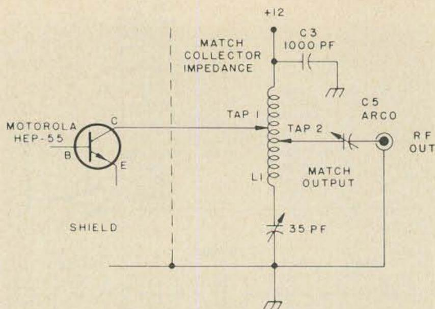
Fig. 6. Collector and output matching.
