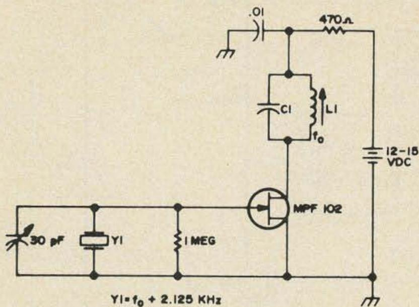
Crystal oscillator for receiver direct conversion. This oscillator will beat against an incoming signal and stay right on frequency even though your receiver may drift a bit. Great for RTTY autostart, net operation, and fixed frequency biz. Circuit courtesy W9ZTK, W9YPS and the RTTY Journal, Box 837, Royal Oak MI 48068. Crystal frequency = net frequency + 2.125 kHz for TT autostart. A 7075 surplus FT2243 crystal can be ground up a couple of kHz so the end result will be autostart on 7075 kHz.
