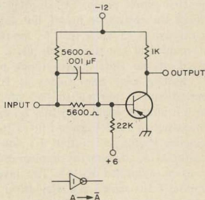
Fig. 15. Typical inverter.
