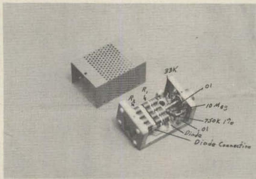
Parts layout and interior view of Dummy Load —
