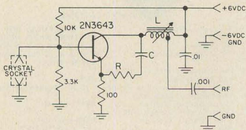
Fig. 2. Layout and schematic, OX-oscillator.
