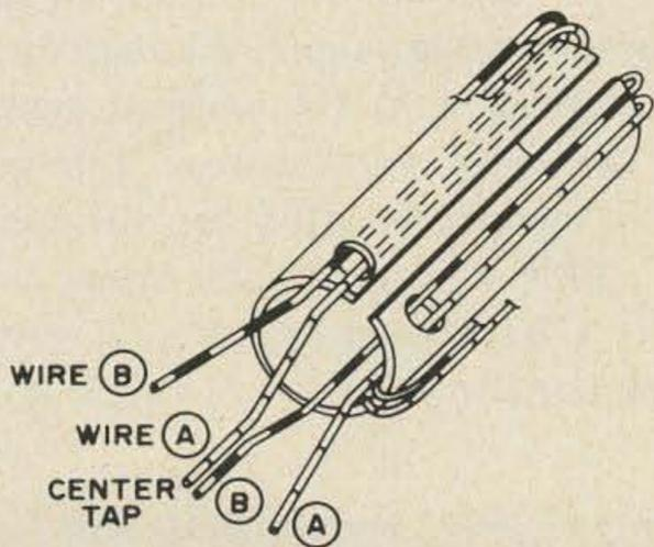
Fig. 3. L1 construction is on 2 in. long RG-8/U casing; 17 turns (lengthwise) of 28-gauge enamel wire.
